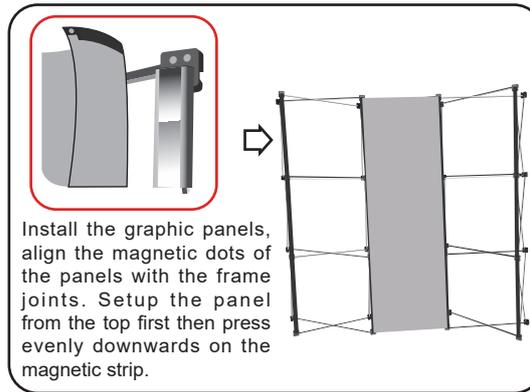
Install the graphic panels, align the magnetic dots of the panels with the frame joints. Setup the panel from the top first then press evenly downwards on the magnetic strip.
