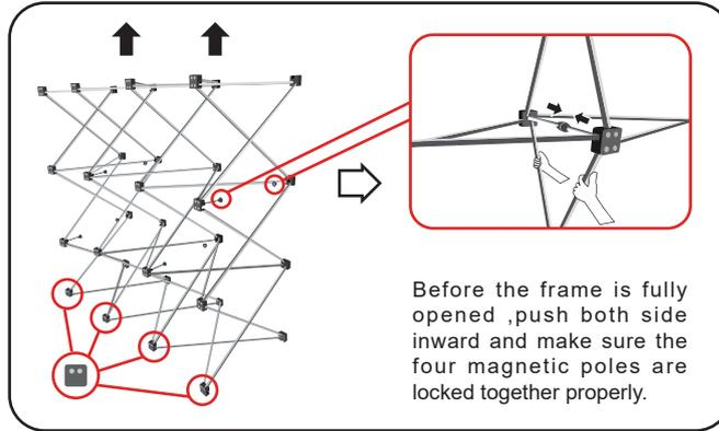
2. Grab two of the poles and gently pull the frame upward.
