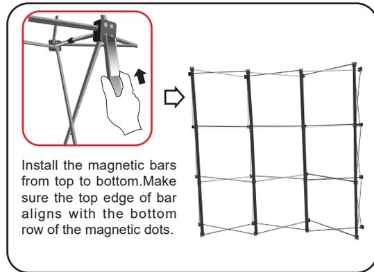
Install the magnetic bars from top to bottom. Make sure the top edge of bar aligns with the bottom row of the magnetic dots.
