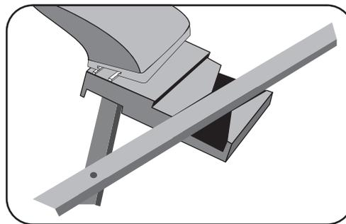
8. Slide the two spot lights on the top cross joint of the frame.
